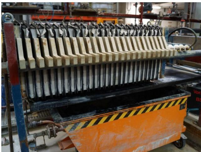
Photograph shows filter press for dewatering solids on wastewater treatment plant.
