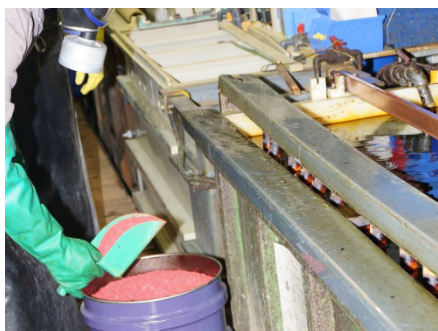
This photo shows adjustment of bath with chromium trioxide.
