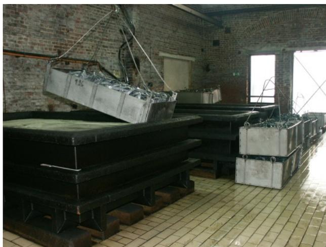
Photographs show (left) racks of parts immersed in a surface treatment bath, (right) a basket of parts being removed from a surface treatment bath. The basket is tilted to allow better draining and to reduce dragout of process solution to the rinse tank.
