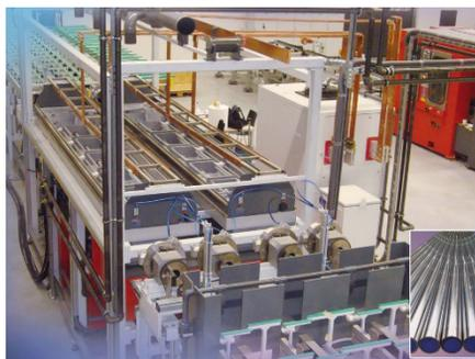
Photographs show covered tanks used in rotogravure plating and continuous plating of hydraulic bars.
