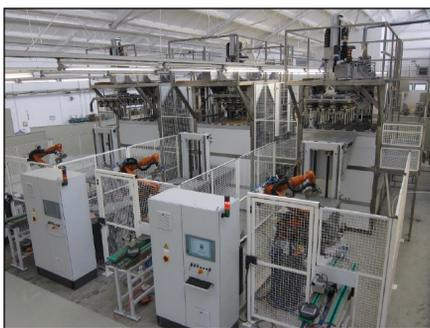
Photographs show closed reactor cells used in plating of piston rods and engine valves.
